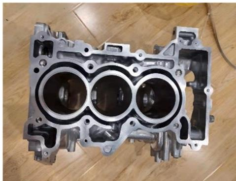
(a) Top surface of a cylinder block
